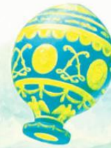
Airship designed by Sir George Cayley (1773-1857), greatest of all early aeronautical pioneers and discoverer of the basic principles of both lighter than air and heavier than air flight. The design is a true airship, a steerable balloon with engine-driven propeller.
