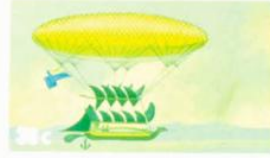
Airship designed by Sir George Cayley (1773-1857), greatest of all early aeronautical pioneers and discoverer of the basic principles of both lighter than air and heavier than air flight. The design is a true airship, a steerable balloon with engine driven propeller.
