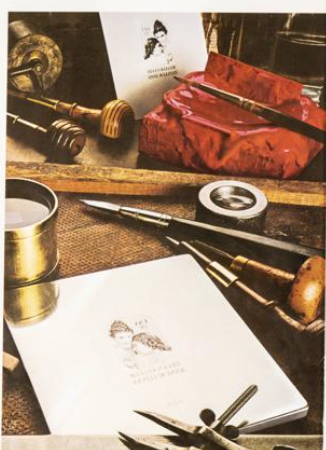
The Engraving The original hand engraved steel die... after six weeks of careful labor. Summertime is the engraving, a photo reduction of the original drawing by artist Paul Cella, and his expert wood during the etching process and engraver's tools—wood-handled galleys and a black-handled hammer.
